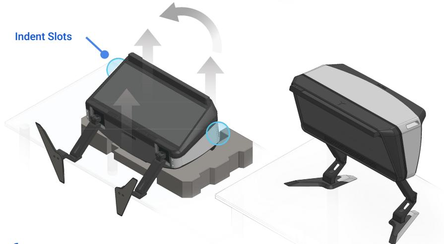
**6.** After securely attaching the legs and feet, gently tip the unit up using the indent slots shown in the blue circle, then lift it up by holding the two bottom sides, and place it on the table upright. (Recommend **two** people for this step.)
