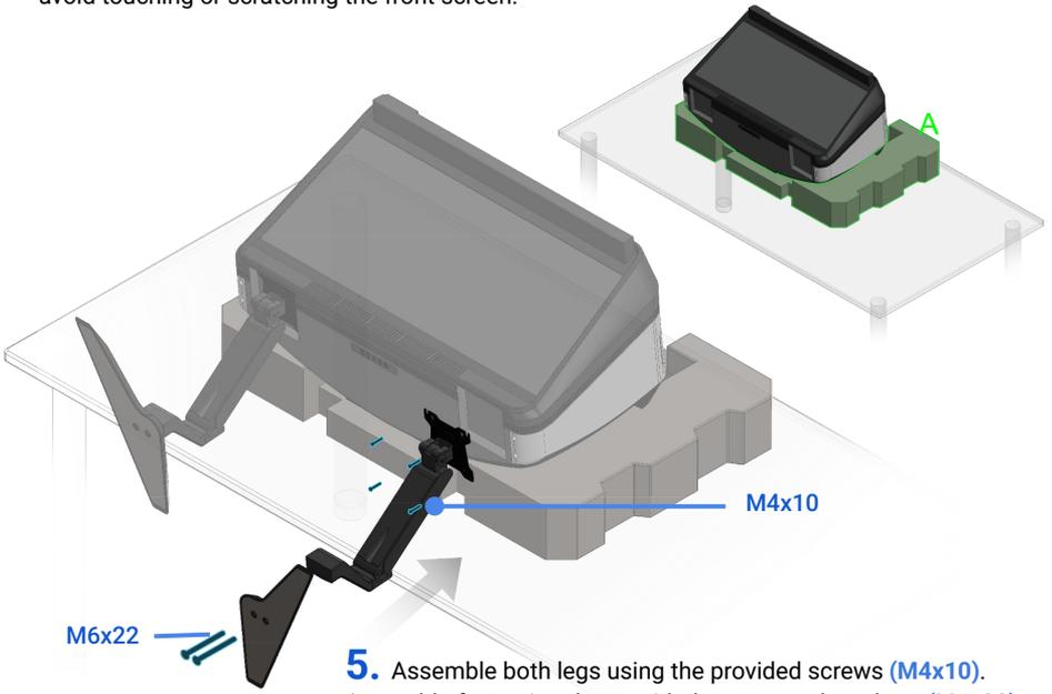
**5.** Assemble both legs using the provided screws (M4x10). Assemble feet using the provided screws and washers (M6x22).
